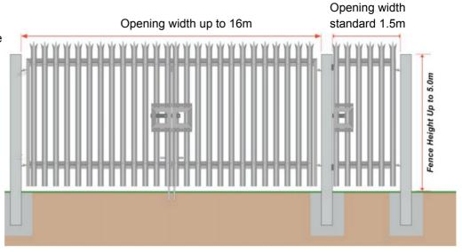
Palisade gates are available in a range of standard heights and specifications to match the style of fencing. Suitable for entrance widths up to 1.6m, with wider entrances normally requiring a sliding gate. The gates can be galvanised or powder-coated in any colour, plus company logos added.
