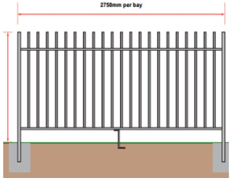
Available in heights from 1000mm to 3.0m, the railings are hot dip galvanised as standard plus we also offer a wide range of polyester powder coated finishes.
