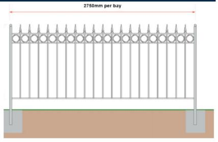
Available hot dipped galvanised or coated polyester powder coated in any colour. Height up to 3.0m.
