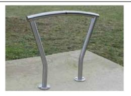
The PROCTER Cycle Stand is a shaped tubular cycle stand. The design allows the frame of the bicy-cle to be secured by the users own security lock. The Cycle Stand is suitable for securing two bicy-cles. The Cycle Stand is available in galvanised steel, Grade 304 and Grade 316 Stainless Steel, with ragged feet for casting into new concrete or flanged feet for bolting to an existing surface.
