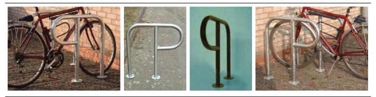
This PROCTER Cycle Stand is a P shaped tubular stand, designed to provide cyclists with a secure stand for locking their cycles. The design allows the frame of the bicycle to be secured by the users own security lock. Suitable for securing two bicycles. The Cycle Stand is available in both galvanised and stainless steel, with ragged feet for casting into new concrete or flanged feet for bolting to an existing surface.
