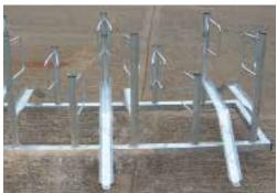
The PROCTER Cycle Rack is a floor mounted cycle rack based upon the Holder. The cycle rack offers an extremely high double sided cycle parking density. The High and Low holders combined ensure that cycles are parked only 170mm apart (typical parking distance for a Sheffield Cycle Stand is 500mm). The high Holders, which incorporate Ramps are arranged in opposite facing pairs, as are the low holders, this combination ensures that all holders can accomdate bicycles at the same time.
