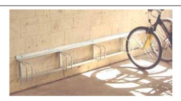
The PROCTER Cycle Rack is a wall mounted cycle rack based upon the Holder. The Cycle Rack is available in Racks for 3 or 5 cycles, but can be manufactured to suit any number of cycles if re-quired. Each individual holder is based on the Cycle Holder, with each holder at 610mm centres. The Cycle Rack is designed to be bolted to a suitable concrete or brick wall.
