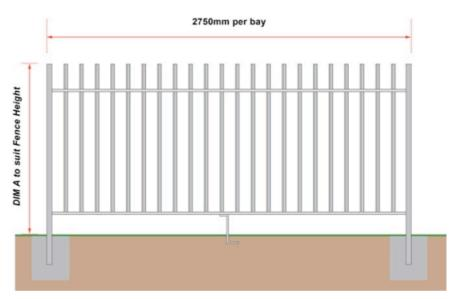
As standard, the railings and posts are galvanised but we also offer a wide range or polyester coated finishes. Height is typically from 450mm to 3m.
